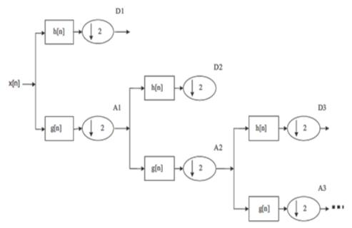
Figure 3. Decomposition with sub-bands by DWT method [12]
