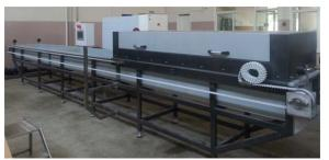
Figure1. Laboratory prototype of microwave oven
