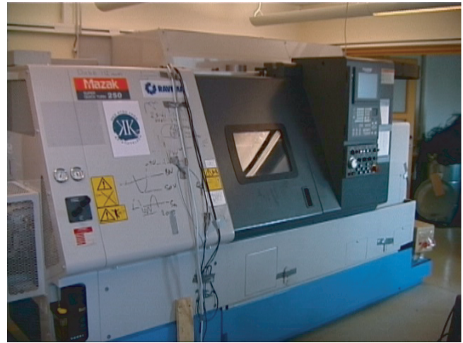
Fig. 1. Figure shows the CNC equipment Mazak SUPER QUICK TURN used in the experiments
