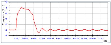
Figure 8. Frequency variation for load shedding, % 100
