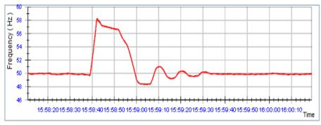
Figure 7. Frequency variation for load shedding, % 50
