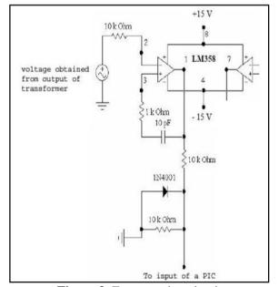
Figure 3. Zero crossing circuit
