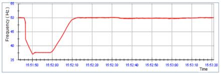
Figure 6. Frequency variation for loading, % 100
