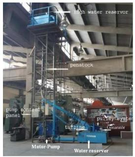
Figure 2. hydro-mechanical section general appearance.
