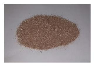
Fig. 2. Vermiculite (Super Fine) used in Experiments
