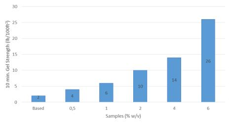
Fig. 6. Analysis results of 10 min. gel strength
