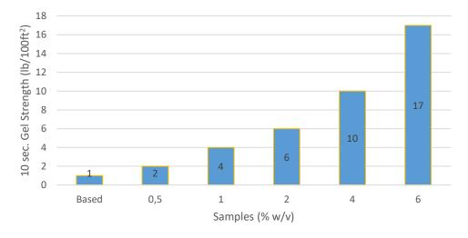
Fig. 5. Analysis results of 10 sec. gel strength
