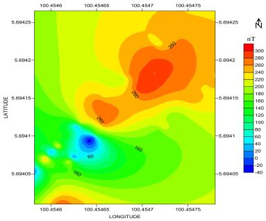
Figure 7. Magnetic Residual Contour Map
