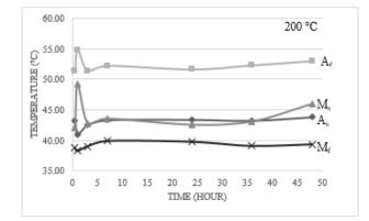
Figure 1. Comparison of transformation temperatures for aged samples at 200  $^{\circ}\mathrm{C}$
