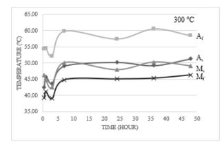
Figure 2. Comparison of transformation temperatures for aged samples at 300 °C.
