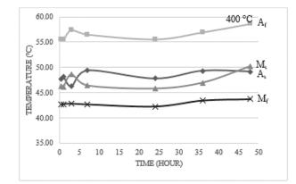
Figure 3. Comparison of transformation temperatures for aged samples at 400 °C.
