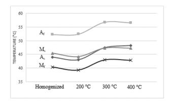
Figure 4. Comparison of mean values of the transformation temperatures.
