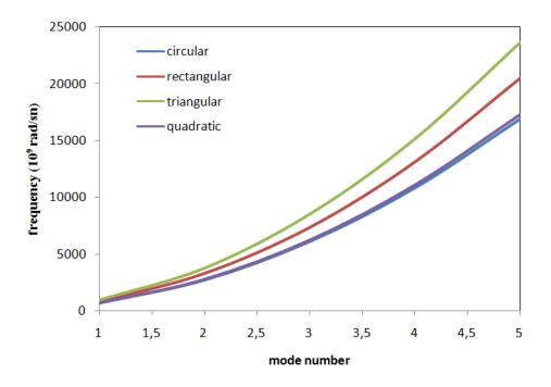
Fig. 1. Frequency values for different cross-sections
