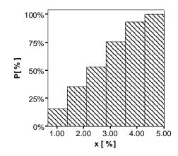
Figure 8. Percentage (P) of estimated discharge with an error not greater than  $\pm(x)$  %
