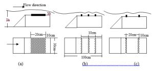
**Figure 2.** Models of (2mm and 6mm) stone roughness distribution; (a) Full, (b) three rows, (c) two rows
