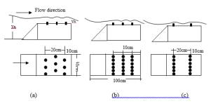
**Figure 3.** Models of (10mm) wood Roughness distribution; Zigzag, (b) three rows, (c) two rows
