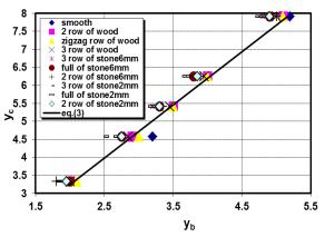
**Figure 5.** The relation between brink and critical depths measured for all cases and computed using eq. (3).
