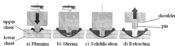
**Figure 1.** A schematic illustration of the FSSW process [10].
