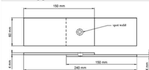
Figure 2: Configuration of the lap-shear test specimen.
