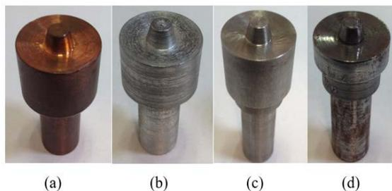
Figure 3. FSSW tools: (a) Copper (Cu), (b) SAE 1050 steel (St), (c) Stainless steel (SS), (d) Aluminum 1050 (Al)
