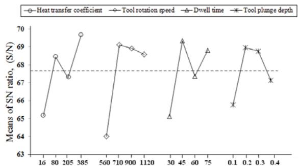
**Figure 5.** The mean S/N response graph for weld strength.
