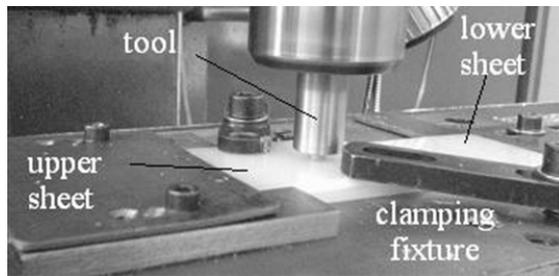
Figure 2. A properly designed clamping fixture.
