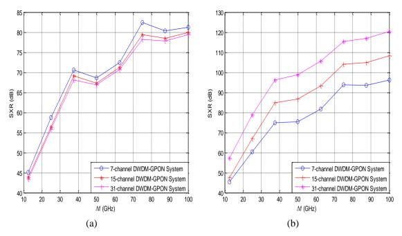
Figure 6: SXR-channel spacing value variations in center downlink channels of 7-, 15- and 31- channel DWDM-GPON systems due to the (a) single impact of FWM (b) combined impact of SRS and FWM
