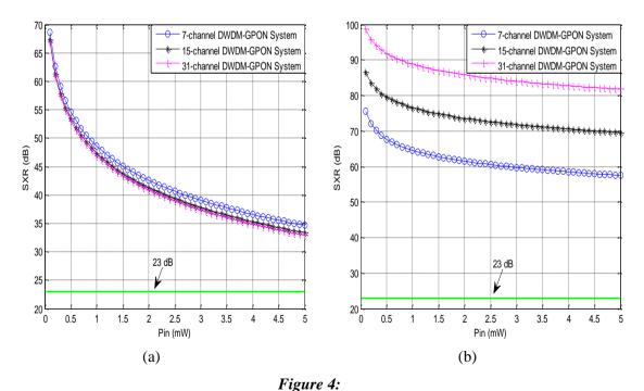
SXR-channel input power variations in center downlink channels of 7-, 15- and 31-channel DWDM-GPON systems that have 50 GHz channel spacing values due to the (a) single impact of FWM (b) combined impact of SRS and FWM
