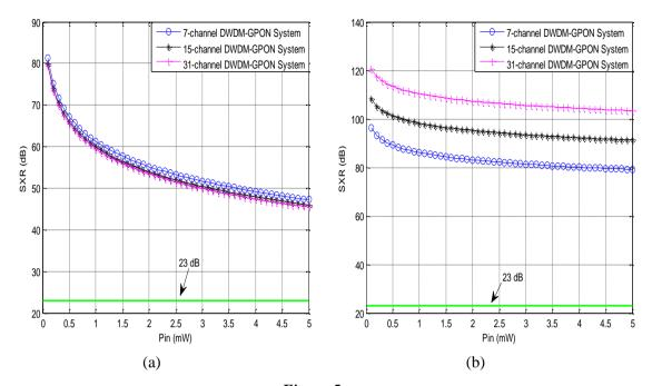
Figure 5: SXR-channel input power variations in center downlink channels of 7-, 15- and 31-channel DWDM-GPON systems that have 100 GHz channel spacing values due to the (a) single impact of FWM (b) combined impact of SRS and FWM
