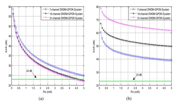
*Figure 3:* SXR-channel input power variations in center downlink channels of 7-, 15- and 31-channel DWDM-GPON systems that have 25 GHz channel spacing values due to the (a) single impact of FWM (b) combined impact of SRS and FWM
