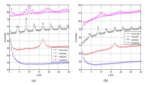
Figure 8: SXR-channel length variations in center downlink channels of 15-channel DWDM-GPON systems for the channel length range of 1-30 km and channel spacing values of 12.5 GHz, 25 GHz, 50 GHz and 100 GHz due to the (a) single impact of FWM (b) combined impact of SRS and FWM
