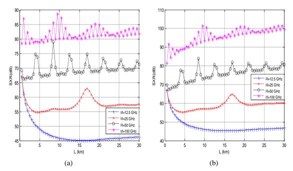
Figure 7: SXR-channel length variations in center downlink channels of 7-channel DWDM-GPON systems for the channel length range of 1-30 km and channel spacing values of 12.5 GHz, 25 GHz, 50 GHz and 100 GHz due to the (a) single impact of FWM (b) combined impact of SRS and FWM
