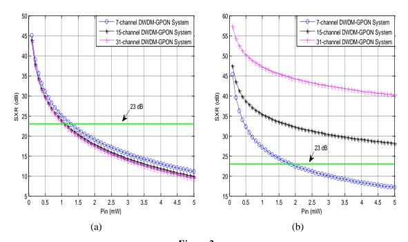
Figure 2: SXR-channel input power variations in center downlink channels of 7-, 15- and 31-channel DWDM-GPON systems that have 12.5 GHz channel spacing values due to the (a) single impact of FWM (b) combined impact of SRS and FWM
