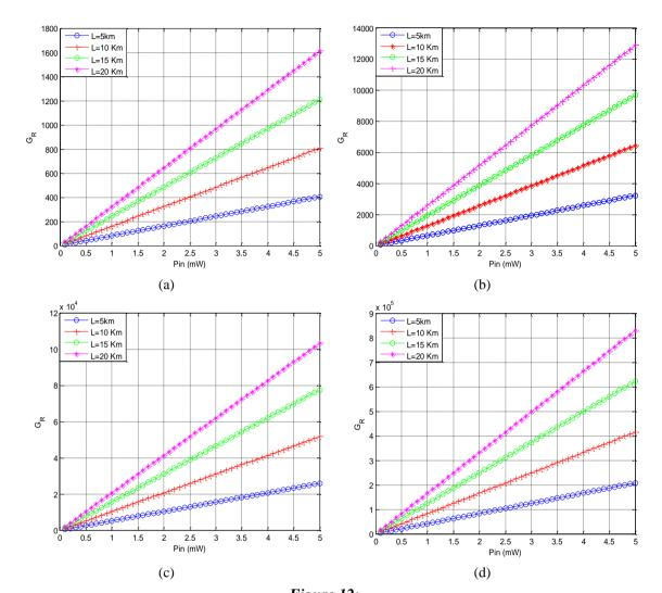
Figure 12:G<sub>R</sub>-channel input power variations in center downlink channels of31-channel DWDM-GPON systems at different channel lengths for channel spacing values of(a)12.5 GHz(b) 25 GHz(c) 50 GHz(d) 100 GHz
