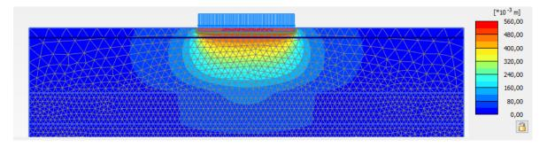
Figure 2. Total Settlement in the FEM model (redrawn after Mungan, 2016).
