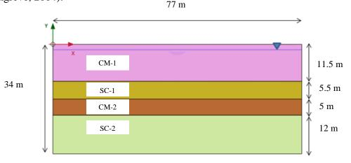
Figure 1. Modelling of soil layers in the FEM software.
