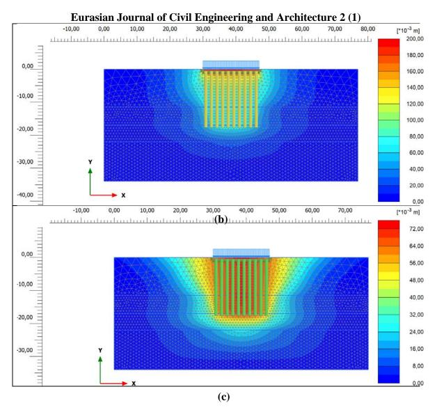
Figure 3. Total displacement in FEM modelling improved with a) RAP, b) JG and c) BP.
