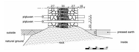
Figure 3. Drawing of the Foundation Type A (Çelik 2009)
