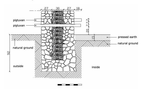
**Figure 5.** Drawing of the Foundation Type B (Çelik 2009)
