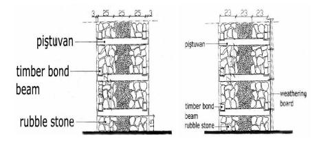
**Figure 9.** Drawing of the Walls with Covering Material (Çelik 2009)
