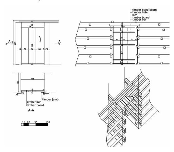
**Figure 8.** Drawing of the Opening Construction (Çelik 2009)
