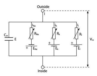
Figure 1. Hodgkin-Huxley electrical model for cell membrane at resting state [REF]
