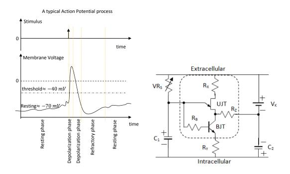
Figure 2 (a) A schematic representation of an Action potential. (b) The electronic model designed to represent cell membrane
