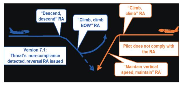
Fig. 2. TCAS RA to avoid collision (EUROCONTROL, 2016)
