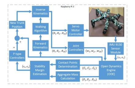
Figure 1. Block Diagram of Walking Control Algorithm
