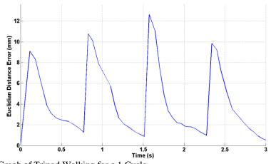
Figure 6. 3 Error Graph of Tripod Walking for a 1 Cycle
