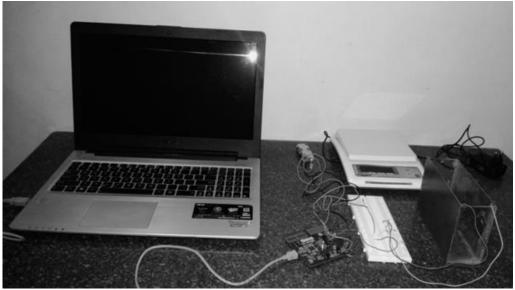
*Figure 4.The arrangement to measure the moisture content of paddy. 1. Personal Computer 2. Bread-Board 3. Evaluation Board 4. Parallel Plate Sensor 5. Electronic Balance*
