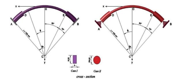
Figure 1. (a) Fix–ended circular stepped beam (b) Pin–ended circular stepped beam
