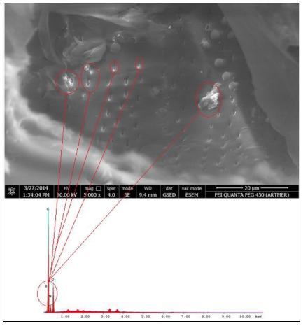
Figure 4. EDAX analysis on the perforation table of the nanoboron impregnated woods.
