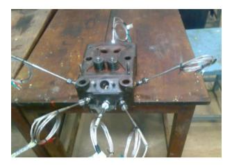
Fig. 6. Cylinder Head with fitted thermocouples
