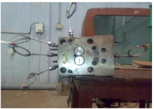
Fig. 5. Cylinder Head with fitted thermocouples
