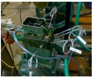
Fig. 7. Kirloskar diesel engine with installed thermocouples
