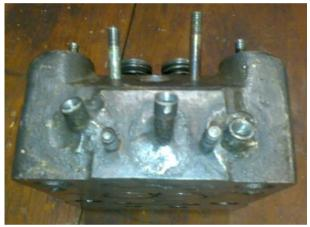
Fig. 4. Cylinder Head with fabricated slaves for fixing thermocouples
