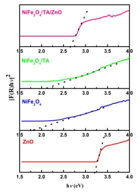
**Figure 3.** The K-M function versus hv curves of the products for band gap energy detection.
