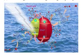
Scheme 1. Schematic representation of photocatalytic degradation for CR via NiFe<sub>2</sub>O<sub>4</sub>/TA/ZnO.
