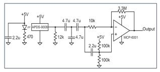
Figure 2. Pulse Sensor Circuit diagram.
