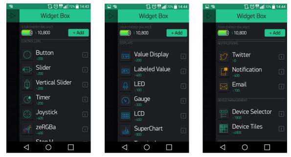
Figure 6. Widget Boxes of the Blynk Interface developer.
