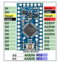
Figure 4. Pinout diagram of Arduino Pro Mini
