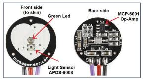
Figure 3. Pulse Sensor front and back sides.
