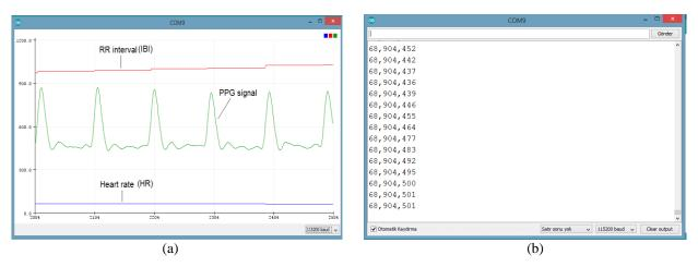
**Figure 13.** (a) Real-time PPG signal obtained from the Arduino IDE Serial Monitor, (b) HR, IBI values and real-time values of the PPG signal.
