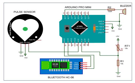
Figure 8. Arduino Pro Mini-based smart health measurement system.
