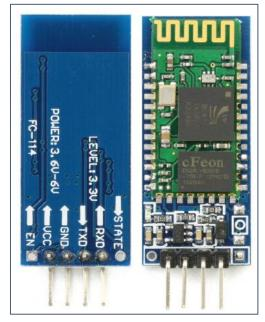
**Figure 5.** The front and back side of the HC-06 Bluetooth module.
