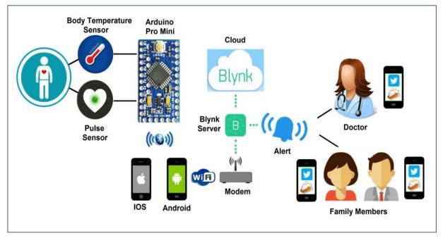
Figure 7. Proposed Structure of the System.
