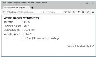
Fig. 7. Vehicle tracking Web interface
