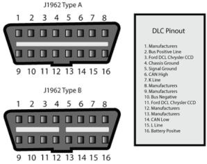
Fig. 1. OBD-II connector wiring [5]
