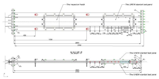
Fig. 1. Pressure drop section with contraction (inlet) and discharge (outlet)
