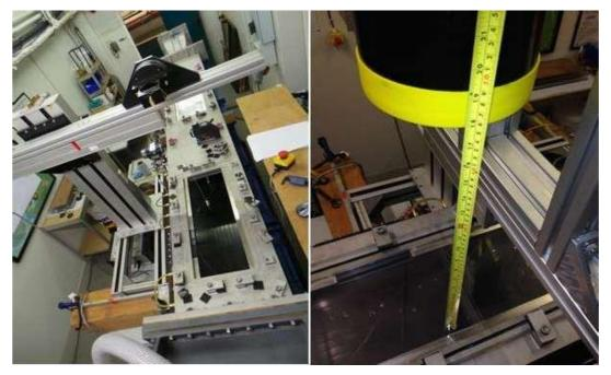
Fig. 5. Traverse arrangement of LDV during calibrations
