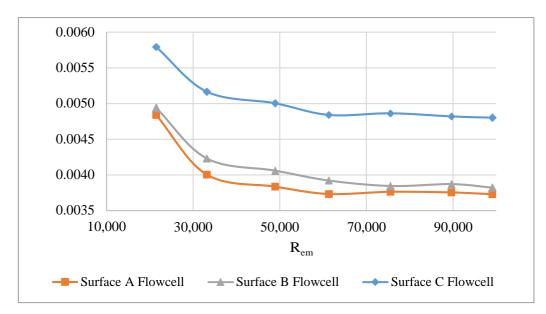
Fig. 9. The comparative friction coefficient of test panels as a function of flow speed.
