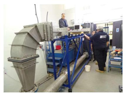
Fig. 2. A view of new test section of the UNEW Flow Cell
