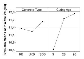
Figure 2. Main effects plot of P wave velocity for S/N ratios
