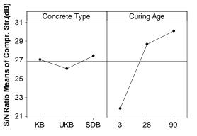
**Figure 3.** Main effects plot of compressive strength for S/N ratios
