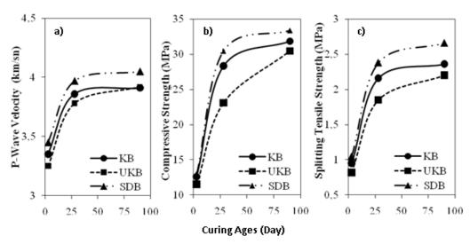
Figure 1. Curing Age-P wave velocity, compressive and splitting tensile strength graphs of concrete series
