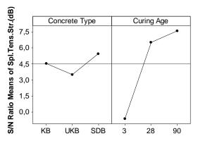
As shown from the Figures 2-4, maximum values for performance characteristics can be obtained by using silica fume in the mix and at 90 days of the curing time. Although UKB series gave experimentally good result at 90 days, it gave statistically minimum values. However, UKB series has very close place to the average line in the Figures 2-4. This result indicates that the fly ash causing a big environmental pollution will be able to use in lightweight concrete mix as a sustainable material.
