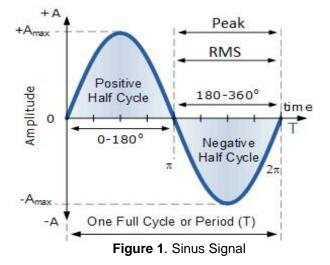
The formulas in the RMS calculation vary to the wave shape formation such as full wave or half wave. Each RMS calculation is based on a different algorithm and provides a true and accurate calculation. Many methods are used to measure the effective values of electrical signals. These methods can be summarized in two titles as comparison and calculation methods (Wey and Huang, 2000).
