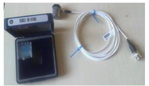
Figure 2. PCB 353B31 vibration sensor
