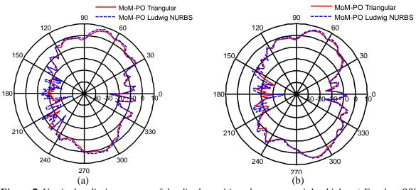
**Figure 7.** Vertical radiation pattern of the dipole positioned over an aerial vehicle; a) For  $\phi = 90^{\circ}$  plane b) For  $\phi = 45^{\circ}$  plane
