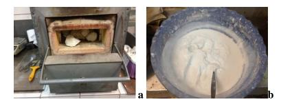
Figure 10. The photographs that show the lime production processes
