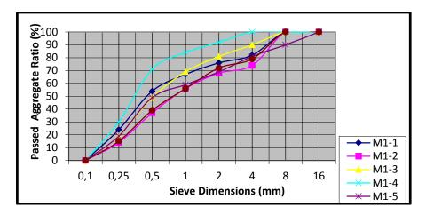
Figure 6. The aggregate granulometry graphs of the samples
