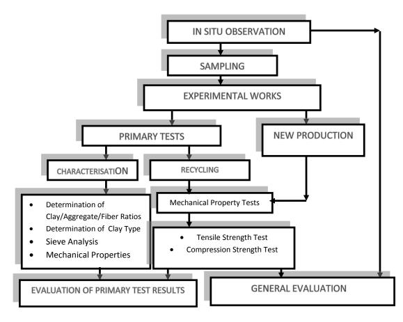
Figure 4. A flow diagram shows the experimental programme
