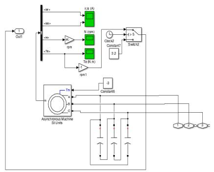
Figure 5. Simulink block diagram for SEIG subsystem
