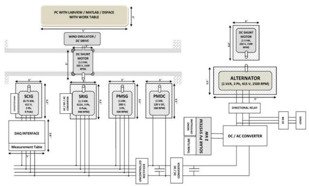
Figure 1. Schematic diagram of wind emulator setup
