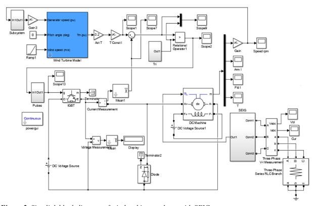
Figure 2. Simulink block diagram of wind turbine emulator with SEIG
