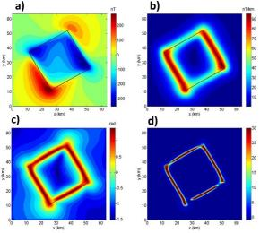
**Figure 2.** Test results of the single prism model (a) Synthetic magnetic anomaly of the single prism model, (b) AS (c) TA, (d) HT<sub>p</sub>, with p = 0.03
