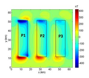
Figure 3. Synthetic magnetic anomaly of the three prisms
