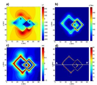
**Figure 5.** Test results of the super positioned two prism models. (a) Synthetic magnetic anomaly, (b) AS (c) TA, (d) HTp, with p = 0.03
