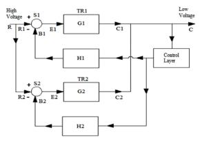
Figure 1. Energy efficiency based dual transformer control
