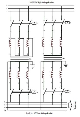
Figure 2. Parallel load transfer of transformers
