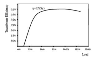
Figure 4. The change of 500-2000 KVA load transformer for  $\eta$ =f(%Sy)
