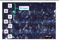
Figure 2. Ti-Al laminated composite (3 bilayer sample).
