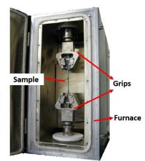
**Figure 4.** Tensile testing machine equipped with a furnace.
