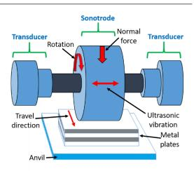
Figure 1. Schematic of the ultrasonic consolidation process.
