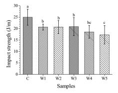
Figure 5. Impact strength values of wood flour-added PVC composites
