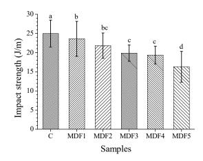
Figure 6. Impact strength values of MDF powder-added PVC composites
