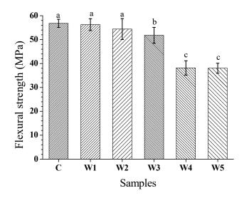
Figure 3. Flexural strength values of wood flour-added PVC composites
