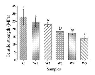
Figure 1. Tensile strength values of wood flour-added PVC composites
