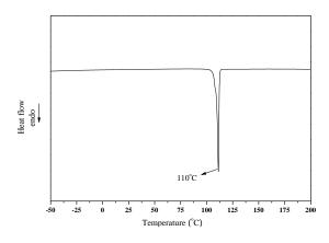
Figure 1: DSC thermogram of the obtained BHET
