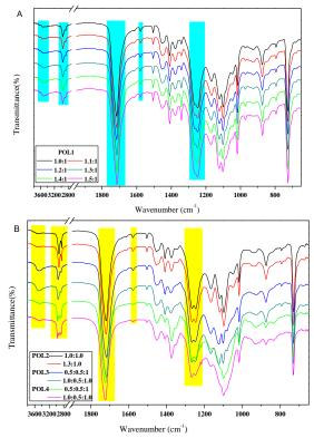
Figure 3. FTIR spectra of polyester polyols (A: POL1 and B: POL2, POL3 and POL4)
