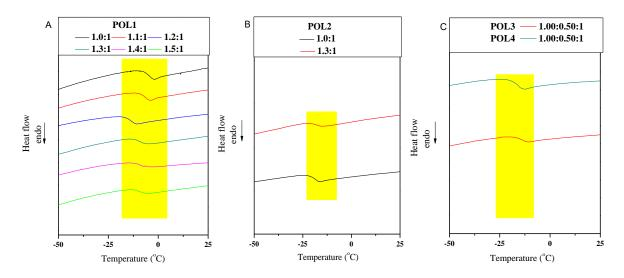
Figure 4. DSC thermograms of polyester polyols
