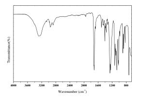
Figure 2. FTIR Spectra of the obtained BHET
