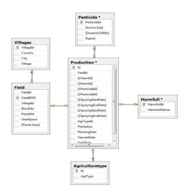
Figure 3. Cotton database diagram
