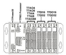
Figure 1. T7RIO remote I/O and its modules.
