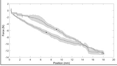
Figure 5. Virtual spring simulation. Solid line and shaded area represent the mean and the standard deviation of the five measurements, respectively. Arrow indicates the direction of movement
