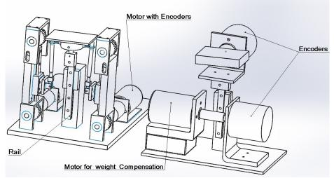
Figure 2. Hardware schematics: (left) haptic interface, (right) input device
