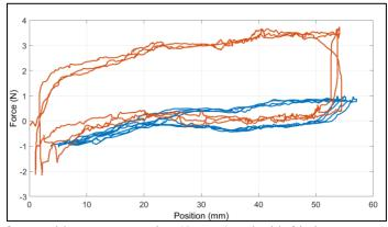
Figure 3. Resistive forces without compensation (Orange) and with friction compensation (Blue)
