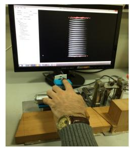
Figure 1. Experimental setup consists of a 2-DOF haptic interface, a 2-DOF input device, a 6-DOF force sensor, two vibration motors, and a virtual environment
