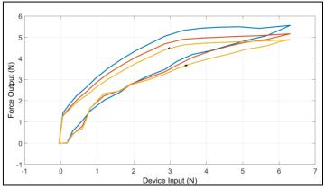
Figure 4. Device input versus force output with friction compensation. Blue, red and orange lines represent the first, second and third trials, respectively
