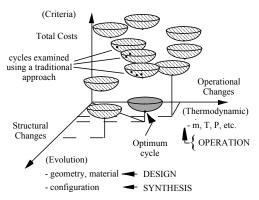
Figure 1. The structural (synthesis-design) and operational (synthesis-operation) space of energy systems (von Spakovsky, 1998).
