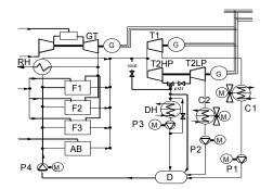
Figure 2. Superconfiguration for the waste incineration cogeneration plant with a gas turbine topping cycle.
