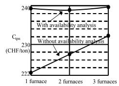
Figure 3. Influence of availability analysis and redundancy on the overall costs of a waste incineration power plant with cogeneration and a topping-cycle.
