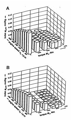
Figure 2. Relative index of total emission of hydrocarbons  $\varphi_{p,HC}$ ; diesel engine - 6C107, *A* - before catalyst, *B* - after catalyst.
