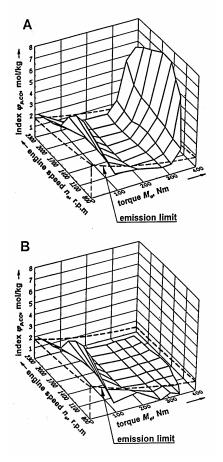
Figure 1. Relative index of emission of carbon monoxide,  $\varphi_{p,CO}$ ; diesel engine - 6C107, *A* - before catalyst, *B* - after catalyst.
