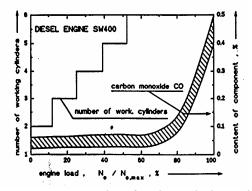
Figure 4. Number of working cylinders and effect of cylinders disconnection on carbon monoxide emission.
