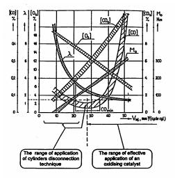
Figure 3. Main ranges of engine work. Effect of specific fuel charge on selected engine parameters.
