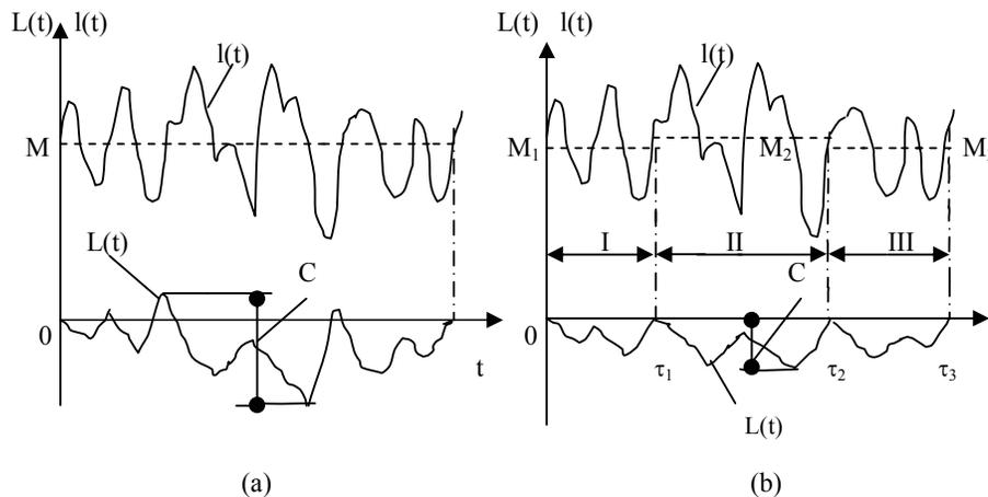
Figure 3. The load graphs of thermal energy system and the integral curves of accumulated thermal energy in different segmentation of the load cycle
