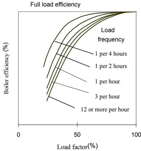
Figure 2. The effect of load fluctuation on the overall efficiency curve
