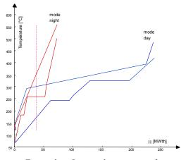
Figure 2. Optimized composites for two extreme operation modes: CC-night and ISCCS-day
