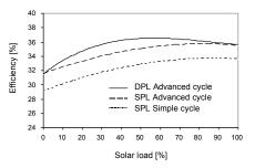
Figure 5. Calculated steam cycle efficiencies
