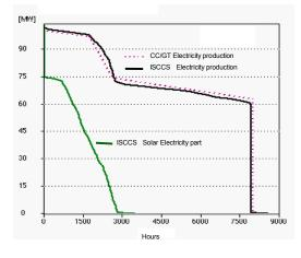
Figure 9. Cumulated curve of the Electricity production
