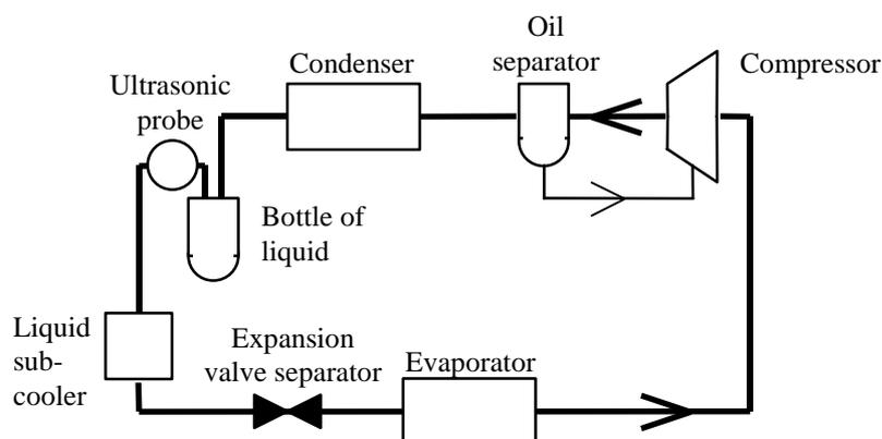
*Figure 4. Simplified diagram of the calorimetric installation.*
