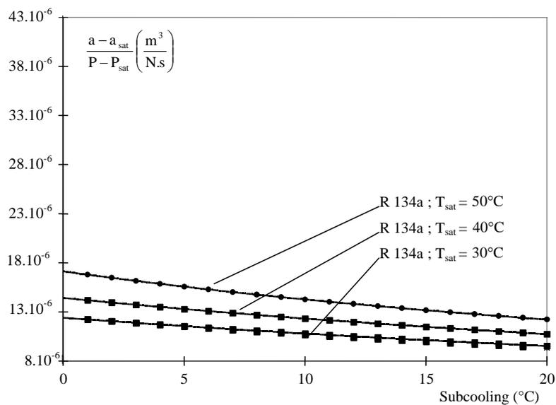
Figure 2. Sensitivity of the speed of sound to subcooling (R 134a)
