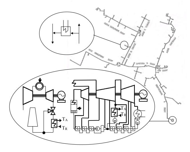
Figure 1. Scheme of the DHN and the two CHP plants
