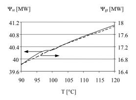
*Figure 5. Thermal energy flow provided by the plants*
