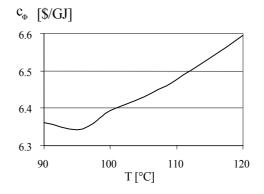
Figure 8. Energy unit cost of the heat supplied
