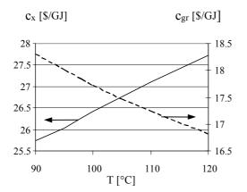
*Figure 6. Unit cost of the thermal exergy provided by the plants*
