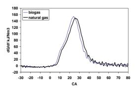
Figure 9. Comparison between natural gas and synthetic biogas heat release rate cycles
