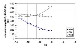
Figure 15. Influence of spark timing on the engine exhaust gas emissions
