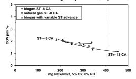
Figure 10. Comparison between natural gas and synthetic biogas, coefficient of variance of pmi
