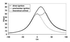
Figure 2. Comparison between direct ignition and prechamber ignition: main chamber pressure cycle for natural gas.
