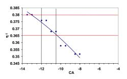
Figure 16. Influence of spark timing on the engine efficiency
