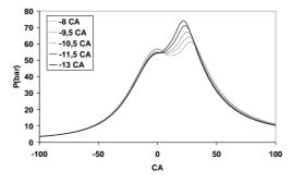
Figure 14. Influence of spark timing on main cylinder pressure cycle
