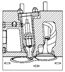
*Figure 1. Combustion prechamber integrated in the cylinder head*
