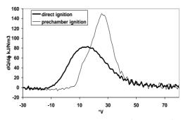
Figure 3. Comparison between direct ignition and prechamber ignition: main chamber heat release rate cycle for natural gas.
