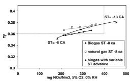
Figure 11. Comparison between natural gas and synthetic biogas, fuel conversion efficiency
