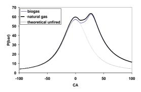
Figure 8. Comparison between natural gas and synthetic biogas pressure cycle
