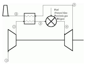
Figure 1. Flowsheet of a recuperated gas turbine
