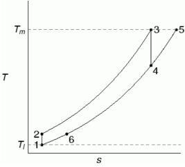
Figure 5. T-s-diagram for the indirectly fired gas turbine cycle
