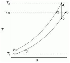
Figure 7. T-s-diagram for the indirectly fired gas turbine cycle with supplementary firing
