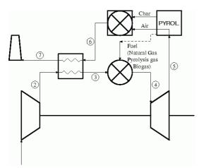
*Figure 6. Flowsheet of an IFGT with supplementary firing*
