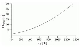
Figure 3. Upper limit of the pressure ratio for a gas turbine with recuperation  $(T_l = 298 \text{ K})$
