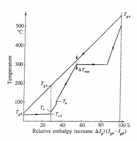
Figure 2. Temperature distribution in the heat recovery boiler of the gas turbine
