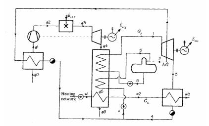
Figure 1. Scheme of the steam-and-gas HP plant; 1-6 states of steam and condensate; g0-g6 states of working fluid in the gas turbine; w1-w3 states of network water,  $\dot{G}_p$ , $\dot{G}_w$  - flow rate of live steam and network water
