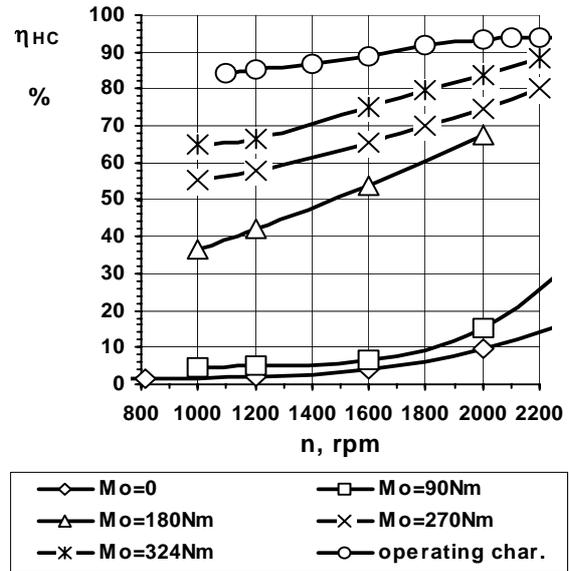
Figure 3. Speed characteristic of HC conversion efficiency for the catalyst SZOP 07 – versus engine speed ( $M_o = idem$ )
