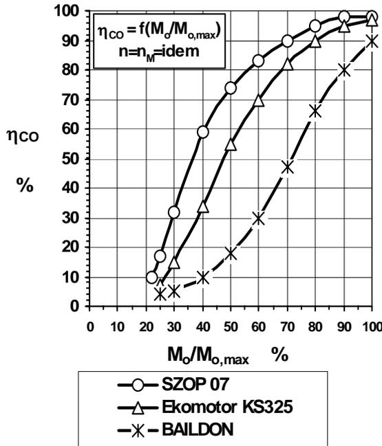
Figure 1. CO conversion efficiency  $\eta_{CO}$  of the oxidation catalytic converters tested – versus engine relative torque (load)
