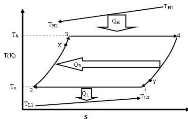
Figure 1. Schematic and T-S diagrams of an irreversible Ericsson heat engine.
