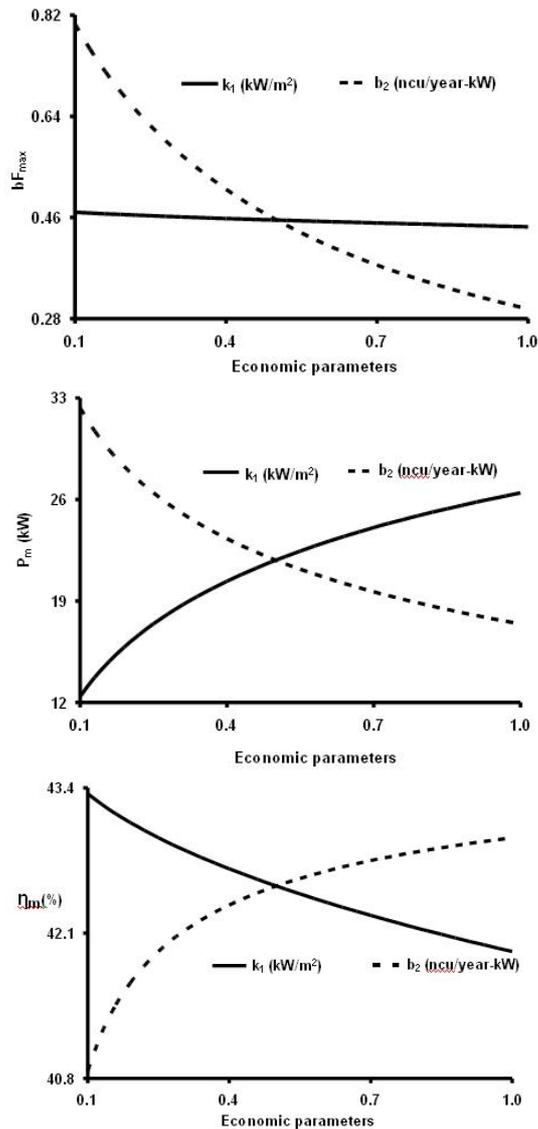
Figure 5. Effects of economic parameters ( $k_1$  and  $b_2$ ) on (a) the maximum objective function, (b) the corresponding power output, and (c) the thermal efficiency, with other parameter values the same as those in Figure 2.
