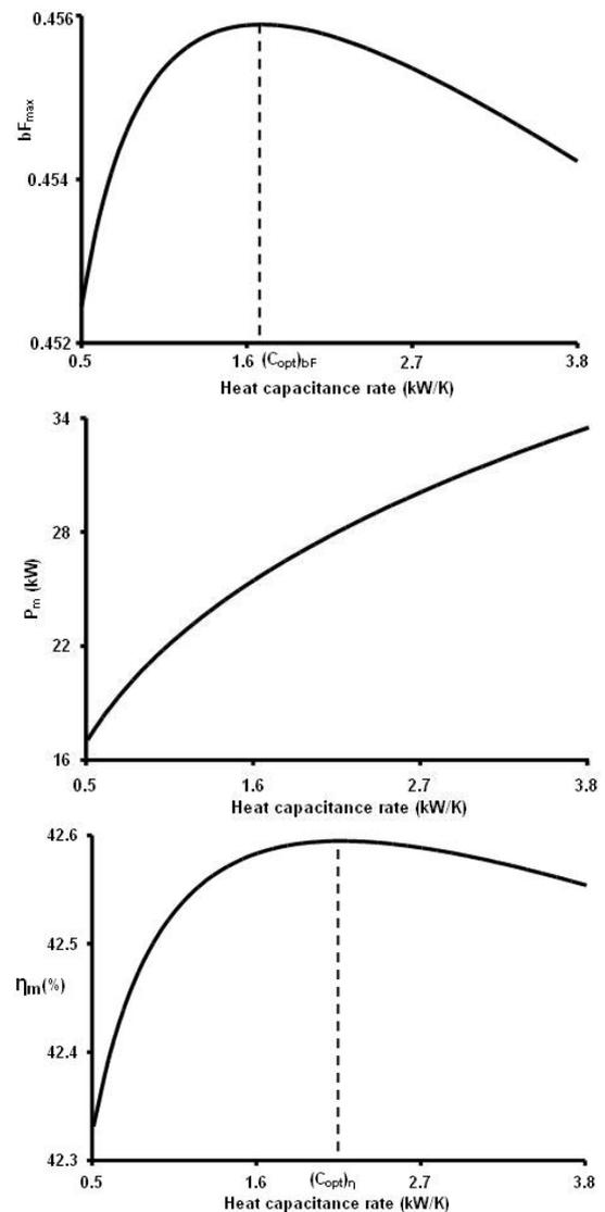
Figure 6. Effects of heat capacitance rate ( $C_H=C_L=C$ ) on (a) the maximum objective function, (b) the corresponding power output, and (c) the thermal efficiency, with other parameter values the same as those in Figure 2.
