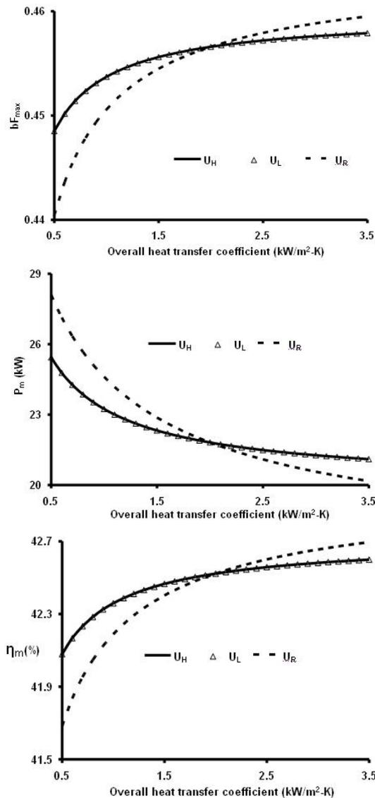
Figure 3. Effects of various overall heat transfer coefficients on (a) the maximum objective function, (b) the corresponding power output, and (c) the thermal efficiency, with other parameter values the same as those in Figure 2.
