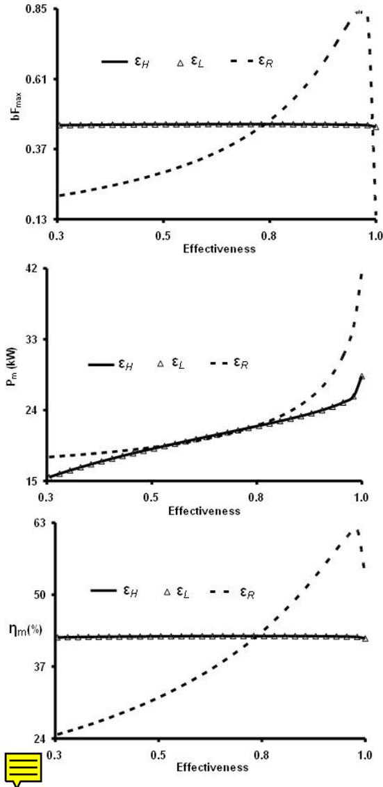
Figure 4. Effects of different effectiveness on (a) the maximum objective function, (b) the corresponding power output, and (c) the thermal efficiency, with other parameter values the same as those in Figure 2.
