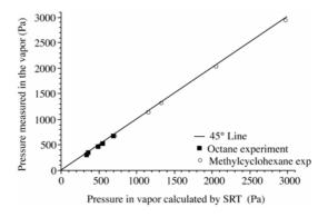
Figure 5. Pressure in the vapor predicted by the SRT expression using measured values of temperature at the interface in the vapor and the liquid and the curvature of the interface at the measured rate of evaporation
