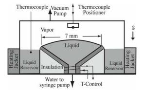
Figure 6. Schematic of the apparatus used in the condensation experiments performed by Ward and Stanga (2001)
