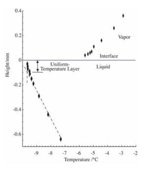
Figure 2. Temperature profile measured in the centerline of the evaporating liquid system (Ward and Duan, 2004)
