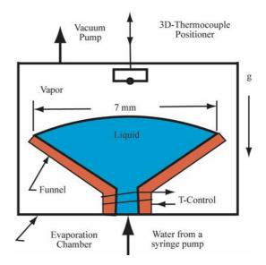
Figure 1. Schematic of the evaporation apparatus used in the experiments of Ward et al. (2004, 1999)
