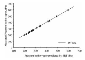
Figure 4. Pressure in the water vapor predicted by the SRT expression using measured values of temperature at the interface in the vapor and the liquid and the curvature of the interface at the measured rate of evaporation. The pressure difference between the predictions and measurements was within the measurements error of 13.3 Pa
