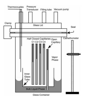
Figure 8. Schematic of the apparatus used in the evaporation studies of Rahimi and Ward (2004)
