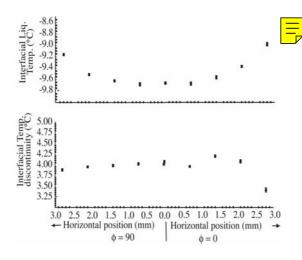
Figure 3. The abscissa indicates the position measured from the centerline in each of two horizontal directions separated by 90°. The upper ordinate gives the interfacial liquid temperature. The lower gives the interfacial temperature discontinuity
