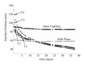
Figure 9. Liquid-vapor interface positions within capillaries and the bulk phase that were measured during the experiment of Rahimi and Ward (2004)
