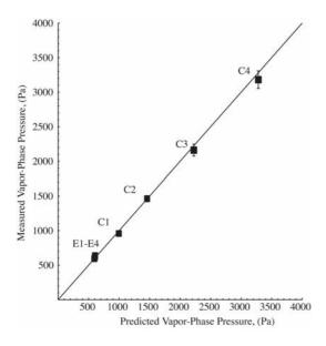
Figure 7. Comparison between the calculated vapor-phase pressure from SRT using the measured rate of evaporation (E1-E4) and condensation (C1-C4) to that measured
